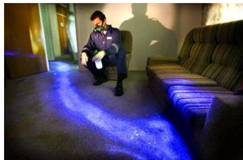
Figure 1: A solution of luminol and hydrogen peroxide being used by a forensic scientist to identify blood at a crime scene [1].
